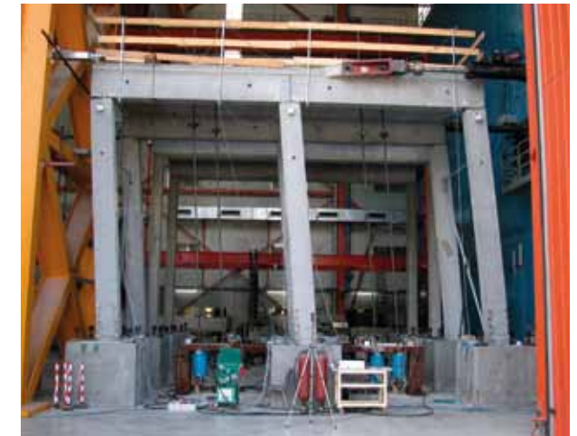
© With kind permission of: Joint Research Centre (ELSA, IPSC), test stand for the simulation of earthquake stress
