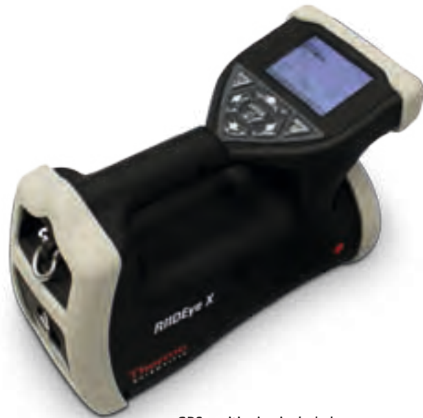
GPS positioning included: an ultramodern measurement device enables mobile nuclide testing in the field
