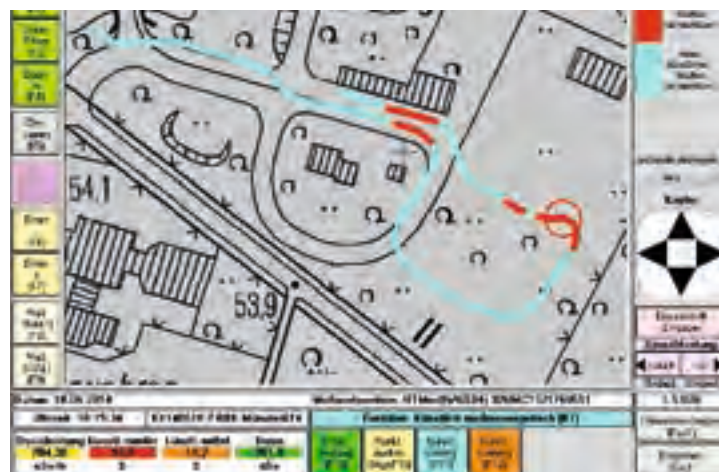
Digitally mapped: radiation intensity in a radioactivity-contaminated area is shown in various colors
