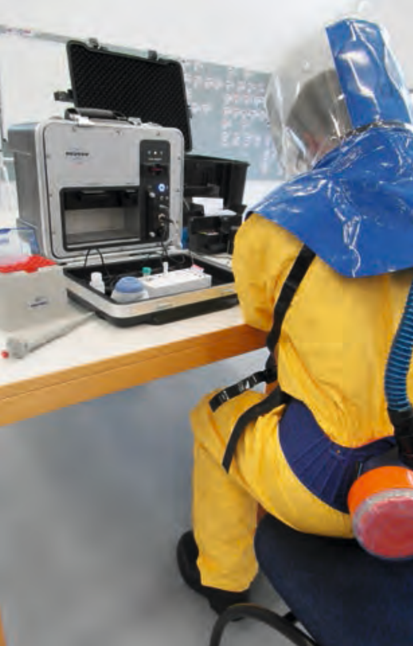
Portable toxin detector identifies biohazards using antibody reactions
