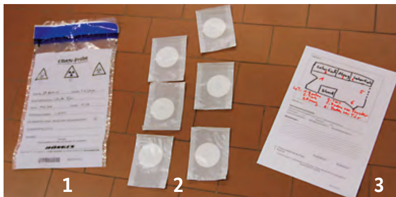
Fig. 22: Components of an RN wipe sample: PE bag (1, decontamination packaging), parchment bag (2, primary packaging) with wipe samples, accompanying form (3)
