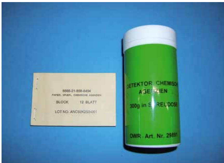
Illustration 7: Example of tracking paper and tracking powder
