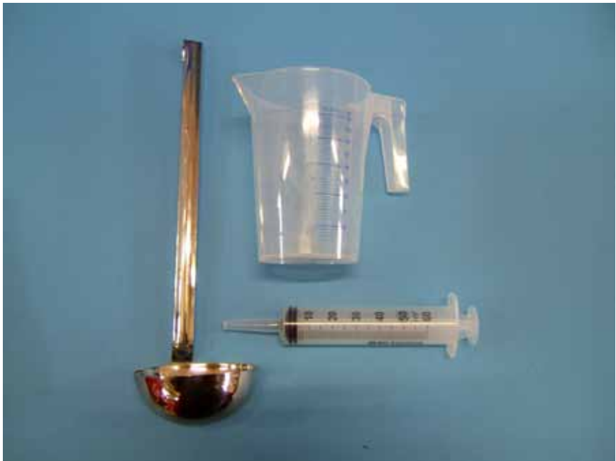
Picture 10: Appropriate sampling tools for taking liquid samples: ladle, measuring jug, syringe
