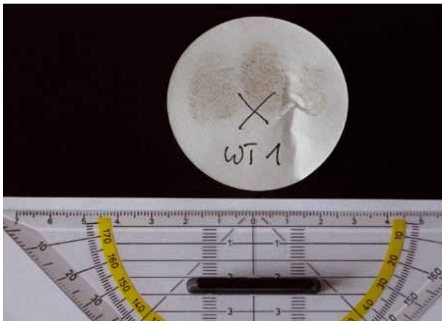
Illustration 11: Wipe sampling with labelled filter and size comparison
