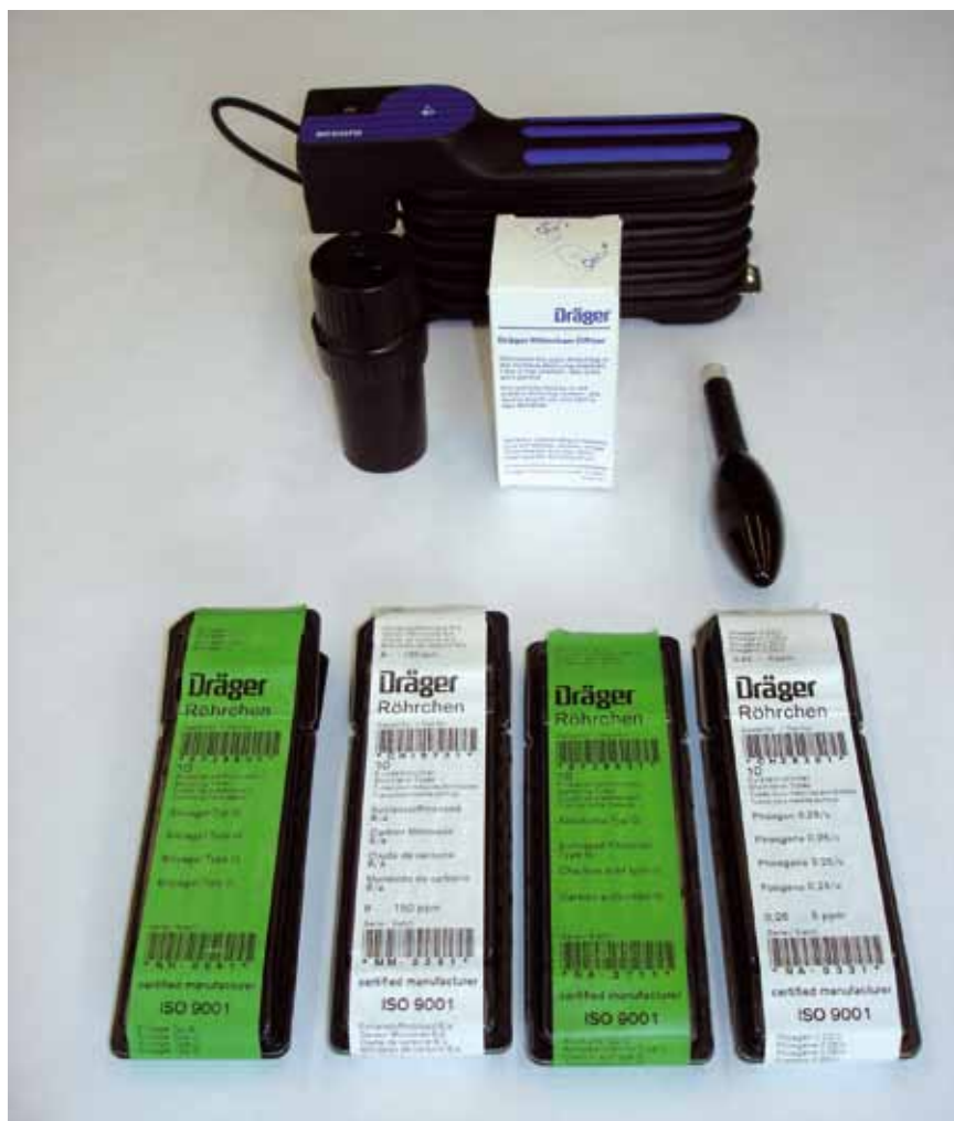
Illustration 6: Example of sorbent tubes with tube opener and manual pump
