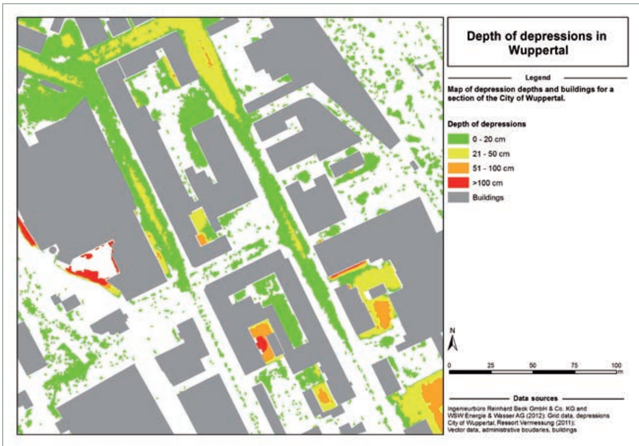
Figure 18: Map of depression depths in a sample section of the City of Wuppertal
