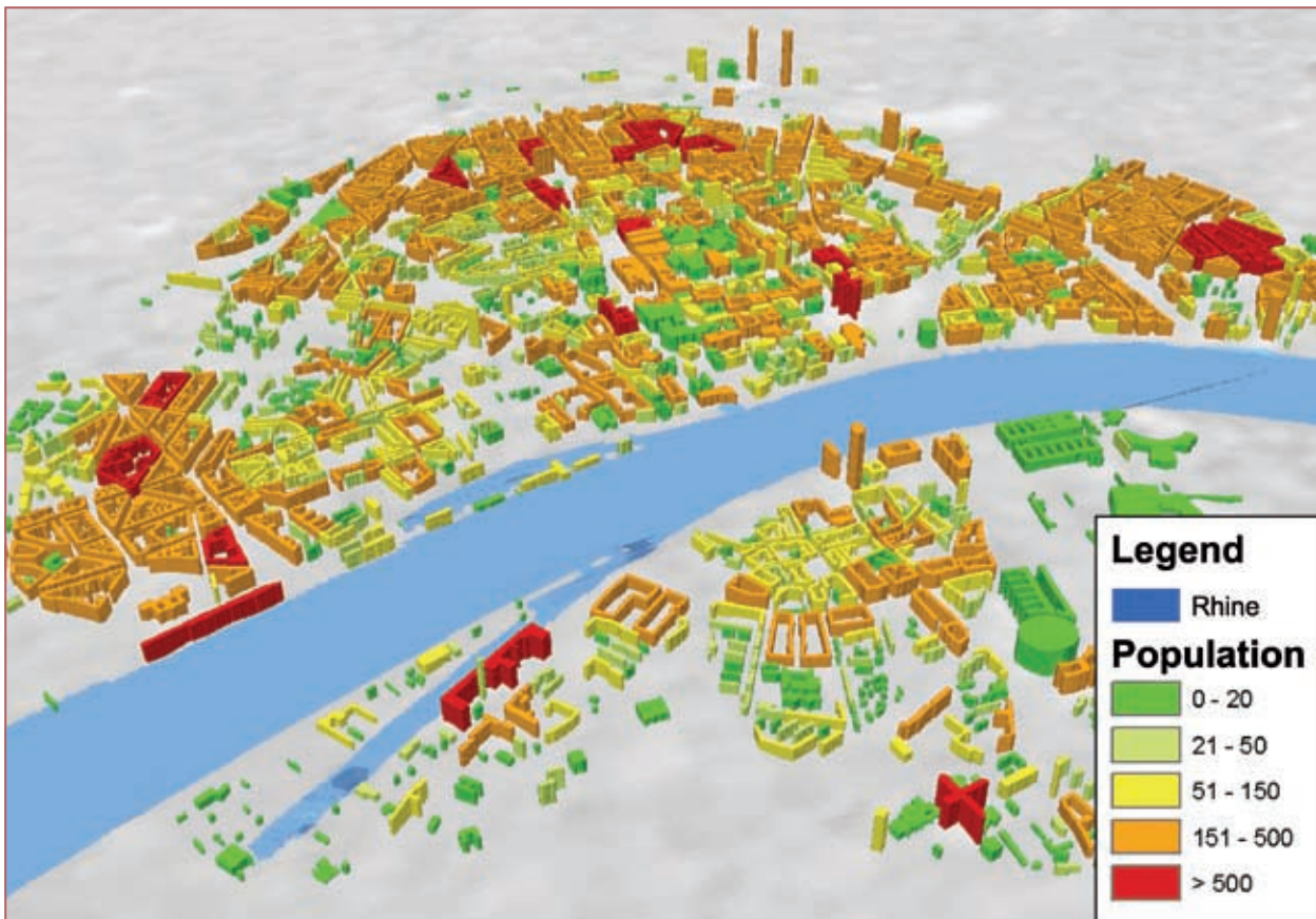
Figure 6.12: Projection of the population distribution onto the three-dimensional city model for the city centre of Cologne
