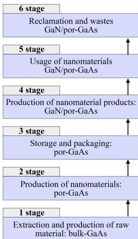
Figure 4 – Life cycle of porous gallium arsenide and gallium nitride based on it
