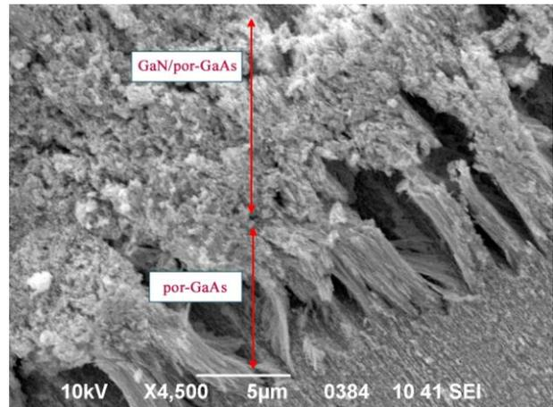
Figure 8 – GaN film is formed at the surface of por-GaAs by the method of radical-beam epitaxy
