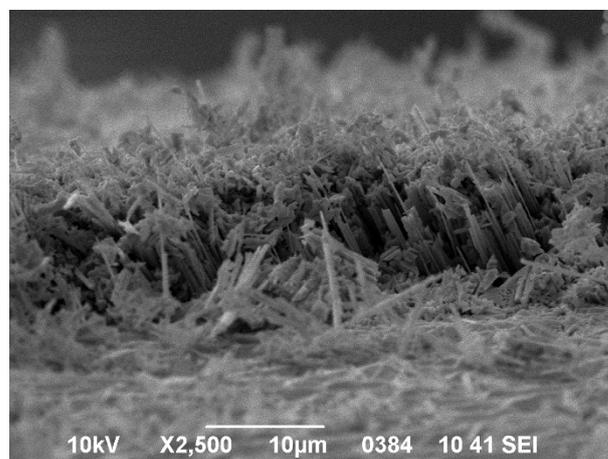
Figure 5 – SEM image of por-GaAs (100): 10 % HCl, j=120 mA/cm<sup>2</sup>, t=5m
