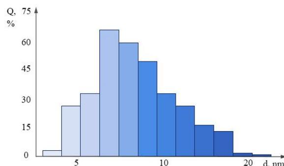
Figure 6 – Distribution of quantum wires by dimensions: Q is the share of particles, %; d – dimensions of particles, nm
