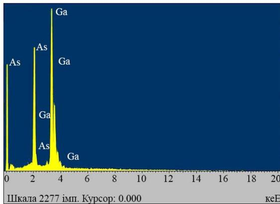
Figure 7 – Chemical composition of elements at the surface of por- GaAs
